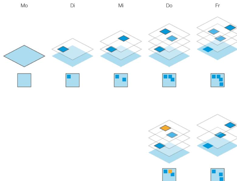
Continuous Snapshots ensure in the Silent Brick System that all changes - including unwanted deletions - can be undone.
