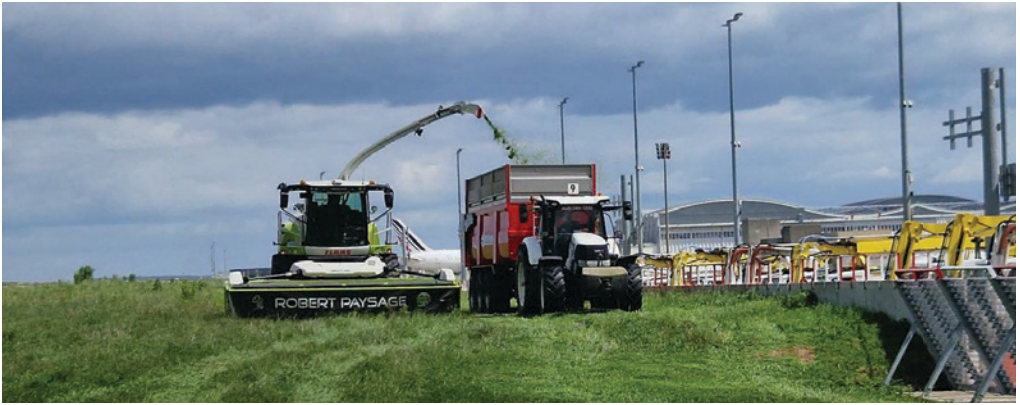
The airside silager triples the yield compared with tractors, while facilitating the methanisation process. © Jonathan Ferreira for Groupe ADP.
