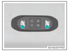
Press a front reading lamp to turn on/off the front reading lamp of concerning side.
