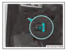
According to the actual vehicle condition, the low beam height can be adjusted via the headlamp leveling roller.
