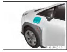
Unlock the vehicle, and press the edge of the charging inlet cap on the left of the vehicle to open the DC charging inlet cap.
