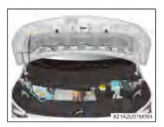
Open the hood, and check the coolant level in the expansion tank as shown. If it is below the "MIN" mark, please fill the expansion tank with coolant to the level between the "MIN" and "MAX" marks in time.
