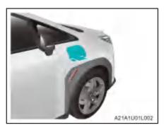
Unlock the vehicle, and press the edge of the charging inlet cap on the right of the vehicle to open the AC charging inlet cap.
