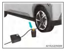
Connect the air pump's connector 3. to the tire sealer bottle.
