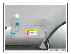
After the sun visor is turned down, disengage the fastening hook (1) and turn the sun visor to the side window to block the dazzling light from the side.
