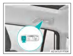
When you press the rear reading lamp switch on both sides, the rear reading lamp of concerning side will be turned on/off.
