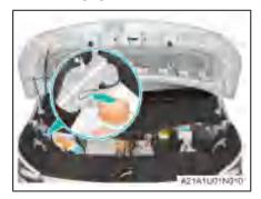
Charger's manual unlocking cable position in National standard charging inlet model
