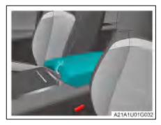
Pull up the central armrest as arrowed, and open the central armrest box.
