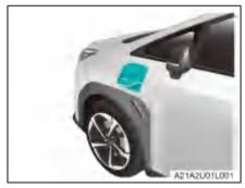
Unlock the vehicle, press the rear edge of the DC charging inlet cap located on the left side of the vehicle to open it.
