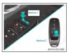
Press the unlocking end of the central locking switch or press and hold the unlocking button of the smart key charger to unlock the charger.
