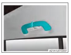
When the vehicle is running fast or on a bumpy road, the safety handrails can be used to keep the body balanced.
