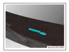
The VIN is pasted at the reserved groove on the lower right of the front windshield.
