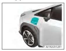
1. Unlock the vehicle, press the rear edge of the AC charging inlet cap located on the left side of the vehicle to open it.
