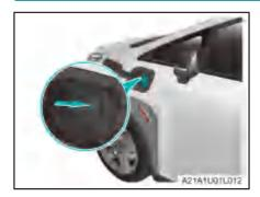
Press the unlocking button on the dust cover of the DC charging inlet, and open the dust cover of the DC charging inlet.
