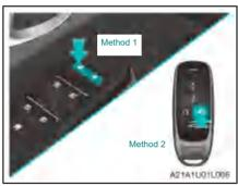
Ends charging actively on demand or stops charging automatically when fully charged.
