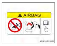
Please follow the warning label on the sun visor: Do not install a child restraint system on the front passenger's seat.
