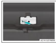
3. Pull the liftgate manual unlocking cable to unlock the liftgate.
