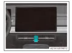
If the vehicle is faulty or involved in a traffic accident, please turn on the hazard warning lamp to alert other vehicles.
