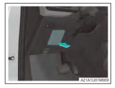
The instrument panel fuse becomes accessible after the driver side lower guard plate assembly is removed.
