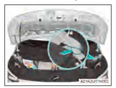
Charger's manual unlocking cable position in European standard charging inlet model
