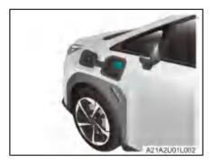
Open the dust cover of the AC charging inlet.
