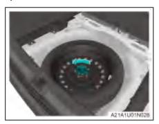
The spare tire is located in the trunk. The spare tire shall not be removed before the trunk carpet and driver's tools are removed.
