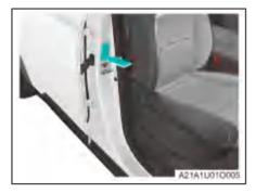
The manufacturer's nameplate is pasted on the near the front door lock catch of B-pillar on the front passenger side.
