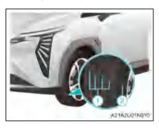
There is a raised "tread wear indicator" ① on the front of the tire. If the tread pattern wears to the indicator surface, the tire can no longer be used safely and must be replaced immediately.
