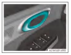
After the door is unlocked, it can be opened by pulling the door inside handle.
