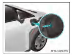
Press the unlocking button on the dust cover of the AC charging inlet, and open the dust cover of the AC charging inlet.
