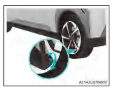
Park the vehicle in a flat and safe 1. place. Remove the tire valve cap.
