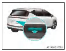
When micro switch with smart key in hand or after the vehicle is unlocked, the liftgate will be unlocked.
