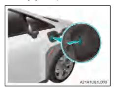
Press the unlocking button on the dust cover of the AC charging inlet, and open the dust cover of the charging inlet.
