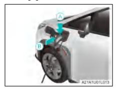
3. Insert the discharger in the direction of arrow B, while pressing the unlocking button of the discharger in the direction of arrow A. All turn signal lamps turn on for quite a bit of time before turning off when the charger is correctly connected, and the instrument's Charger Connected indicator lamp = illuminates.
