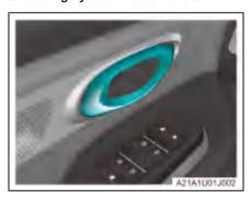
The locked door can be unlocked by pulling the door inside handle.
