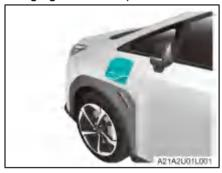
Unlock the vehicle, and press the edge of the charging inlet cap on the left of the vehicle to open the charging inlet cap.
