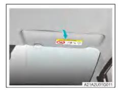
Sun visors are located above the driver's seat and front passenger's seat. Turn down the sun visor to block the dazzling light from the front.
