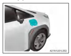
Unlock the vehicle, and press the edge of the charging inlet cap on the left of the vehicle to open the AC charging inlet cap.
