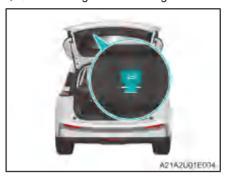
When the liftgate is opened, press the liftgate button, and the liftgate will close automatically.
