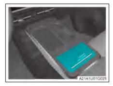
Press the console storage box as arrowed to open it.
