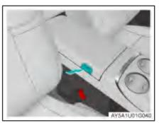
Press the vehicle refrigerator lid's open button to lift the lid and access the refrigerator.
