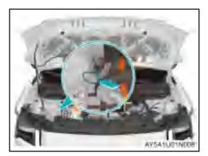
2. Pull the charger manual unlocking cable to unlock the charger.
