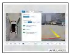
Tap to set soft keys. The system will pop up the settings interface. Trajectory, time of moving out of "P" position, transparent chassis, panoramic view after activation of radars, and panoramic view after activation of turn signal lamps can be set as needed.
