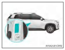
The manufacturer's nameplate is pasted on the near the front door lock catch of B-pillar on the driver side.
