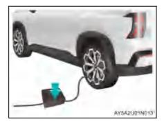
4. Start the vehicle, and turn on the air pump for inflation.
