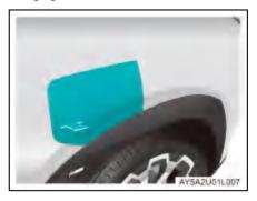
After the vehicle is unlocked, press the rear edge of the charging inlet cap to open the charging inlet cap.
