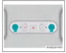
Press a front reading lamp to turn on/off the front reading lamp of concerning side.
