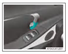
When the door is locked, pull the inner handle of the front door to unlock it.
