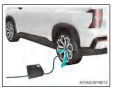
2. Screw the connector of the air pump into the tire valve cap.
