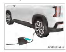
Observe changes in the air pressure gauge. Turn off the air pump to stop inflation when the standard tire pressure is reached.
