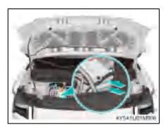
Open the hood, and check the coolant level in the expansion tank. If it is below the "MIN" mark, please fill the expansion tank with coolant to the level between the "MIN" and "MAX" marks in time
