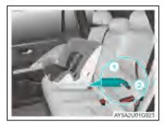
Secure the locking mechanism of the lower part of the child seat ① correctly to the ISOFIX anchorage of the rear seat ②.
