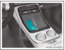
Place a mobile supporting wireless charging in the wireless charging area. To ensure good wireless charging experience, it is suggested the mobile should be close to the rear air outlet of the charging area, and align the mobile charging coil with the charging area shown in the image.
