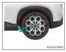
Remove the wheel bolts, and take off the damaged wheel.
