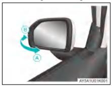
Pull the exterior rearview mirrors toward the rear of the vehicle (arrow A) to manually fold them.
