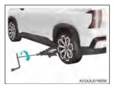
Insert the special wrench for jack into the jack, turn the special wrench for jack clockwise with the wheel bolt wrench, and slowly raise the jack to lift the tire off the ground slightly.
