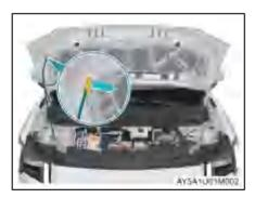
Take out the support bar and insert it into the position as shown in the figure to fix the hood
