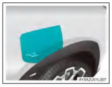
1. Unlock the vehicle, press the rear edge of the charging inlet cap to open it.
