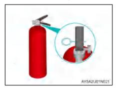
If there is a fire, pull out the safety pin, aim at the root of the flame and press the handle.
