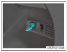
12 V power outlet in the trunk Enter the vehicle, lift the 12 V power outlet cover and connect an electrical consumer at the same time to use the 12 V power supply.
