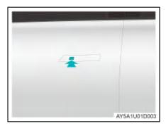
When the vehicle is locked, carrying the smart key and pressing the micro switch will unlock the vehicle.
