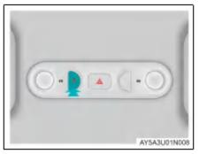
When the vehicle is powered on or in motion, pressing the emergency power off switch will prompt a related message on the instrument panel. At this time, holding the emergency power off switch for a period or pressing the switch three times in quick succession will initiate an emergency power off.
