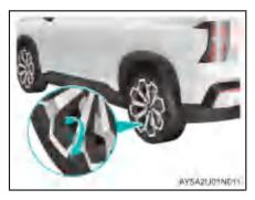
1. Park the vehicle in a flat and safe place. Remove the tire valve cap.
