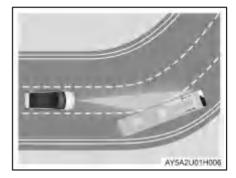
Driving through a curve. During driving through a curve, the sensor may fail to capture the vehicle ahead, or may respond to vehicles in adjacent lanes. In this case, the ACC may make no response to the vehicle ahead or make unnecessary brake. The driver should actively take over the vehicle.
