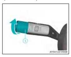
Turn the wiper control knob up or down from the O position, so that the front wiper position icons are aligned with the wiper control knob position reference icons in turn, and the front wiper mode can be selected. The specific control is as follows:
