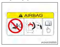
Please follow the warning label on the sun visor: Do not install a rear-facing child restraint system on the front passenger seat.
