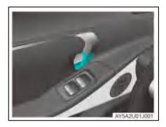
After the door is unlocked, pull the inner handle of the front door to open it.
