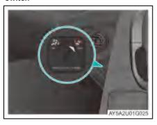
The front passenger airbag suppression switch is on the side of the instrument panel.
