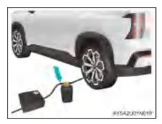
3. Connect the air pump's connector to the tire sealer bottle.
