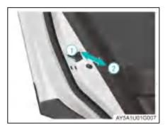
When a child takes a rear seat, please move the switch to locking position before closing the door. At this time, the door cannot be opened from inside, so as to prevent the child from opening the door unexpectedly.
