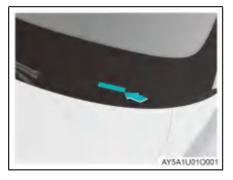
The VIN is pasted at the reserved groove on the lower right of the front windshield.
