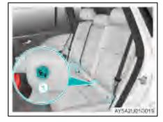
There are four i-Size anchorages provided between the rear seat back and seat cushion for the installation of child seat. Label ① is used to indicate the location of the i-Size anchorage.
