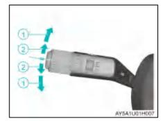
Turn signal: Move the light/wiper control lever to ① position. After you release it, the light/wiper control lever will automatically return and the corresponding side turn signal lamp will flash continuously. After the steering wheel returns, the turn signal lamp will turn off automatically.
