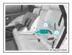
Secure the locking mechanism of the lower part of the child seat ① correctly to the i-Size anchorage of the rear seat ②.
