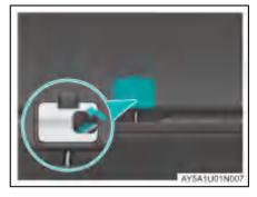
Remove the liftgate emergency unlocking port cover from the liftgate guard plate.
