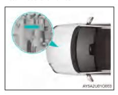
The motor model and number are engraved on the motor housing.
