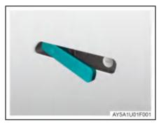
When the vehicle is unlocked, the hidden door handle automatically unfolds and you can open the door by pulling the door handle
