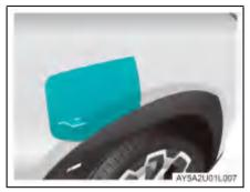
Unlock the vehicle, press the rear edge of the charging inlet cap to open it
