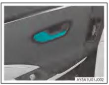
When the door is locked, pull the inner handle of the rear door to unlock the corresponding door.
