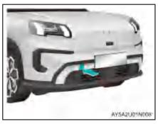
Open the towing cover at the lower right of the front bumper.
