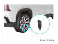
Remove the tire valve cap, align the pressure measuring interface of the digital tire pressure gauge with the tire valve, and then hold it for a period of time, remove the observed reading.
