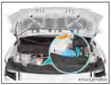
Open the hood, open the washer fluid reservoir cap as arrowed, and check the washer fluid in the reservoir. If the washer fluid level is too low, please add the washer fluid or a mixture of washer fluid and water.
