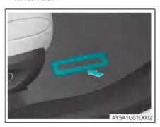
The VIN is engraved at the floor in front of the driver's seat.
