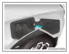
The vehicle charging warning sticker is located on the charging inlet cap.
