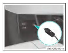
Insert the power plug into the power outlet interface.
