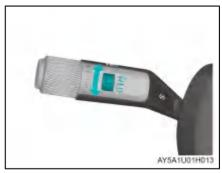
Toggle the rear wiper switch up or down from OFF position to select a wiping mode for the rear wiper. Details are as follows:
