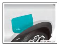
Unlock the vehicle, and press the rear edge of the charging inlet cap to open it.
