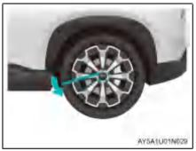
Turn the wheel bolts counterclockwise with the wheel bolt wrench, to loosen them by 1~2 turns.
