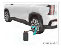
2. Shake the tire sealer and screw its connector into the tire valve cap.
