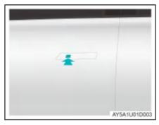
When the driver and passengers exit the vehicle, and the vehicle is not started, all doors are closed, and there is no valid key inside the vehicle, press the micro-switch with the smart key to lock the vehicle.
