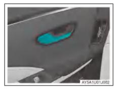
After the door is unlocked, pull the inner handle of the rear door to open it.
