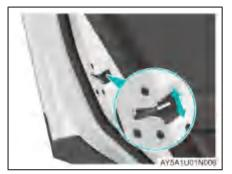
Insert the mechanical key into the keyhole in the door lock, turn the key downward to the locked position, pull out the mechanical key, and close the door to lock the door.
