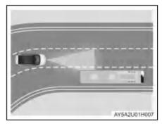
Driving out of a curve. During driving out of a long curve, as ACC will calculate the lane in advance, the radar may respond to the vehicles in adjacent lanes and apply the brake of your vehicle.
