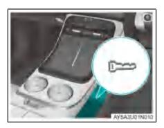
When the battery of smart key runs out or is low, enter the vehicle, place the smart key at the mark, depress the brake pedal and power on the vehicle, and then move the gearshift lever as soon as possible start the vehicle.
