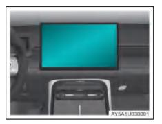
The center console display will show the original image for seconds and start to work, after the whole vehicle is powered on
