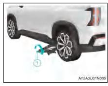
Turn the jack ① clockwise so that the jack is close to the lifting point of the body.
