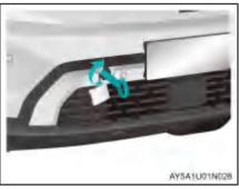
2. Insert the towing hook into the towing port, turn it clockwise and tighten it.
