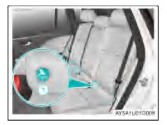
There are four ISOFIX anchorage provided between the rear seat back and the rear seat cushion for installation of child seat. Label ① is used to indicate the position of ISOFIX anchorage.
