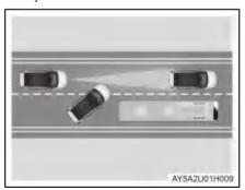
a vehicle in the adjacent lane goes into the ego lane, if it does not enter the detection range, it could not be detected by the sensor, thus resulting in a response lag of ACC.
