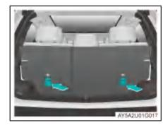
The Top tether anchorage is located on the back of rear outboard seat.
