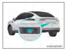
When you press the trunk micro switch with smart key in hand or after the vehicle is unlocked, the trunk lid will automatically open.
