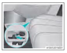
2. Pull the manual unlocking cable to unlock the door.
