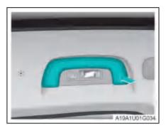
When the vehicle is running fast or on a bumpy road, the safety grips can be used to keep the body balanced.
