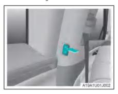
When the doors are locked, press the door opening button on the left/right B-pillar to automatically unlock the left/right gull-wing door. (Models with rear gull-wing doors)
