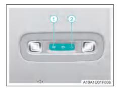
Press the end 1 of the rear reading lamp switch to turn on the rear reading lamp. Press the end 2 of the rear reading lamp switch to turn off the rear reading lamp.
