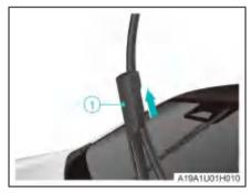
Press the wiper blade lock button 1, and remove the wiper blade in the direction of the arrow.
