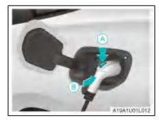
While pressing the button of the charger in the direction of arrow A, insert the charger in the direction of arrow B. After the charger is successfully connected, the vehicle charging indicator lamp stays on in yellow, and the charger indicator lamp on the instrument comes on.
