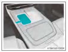
Place a mobile phone that supports wireless charging in the wireless charging area. To ensure a good wireless charging experience, it is recommended to place the phone as close to the air outlet at the rear of the charging area as possible, and align the phone charging coil with the charging icon area.
