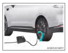
2. Screw the connector of the inflator pump into the tire valve.
