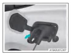
7. Pull out the charger in the direction of the arrow.
