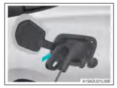
Insert the charger in the direction of the arrow. After the charger is successfully connected, the vehicle charging indicator lamp stays on in yellow, and the charger indicator lamp on the instrument comes on.
