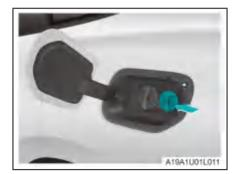
2. Remove the AC charging port dust cap.
