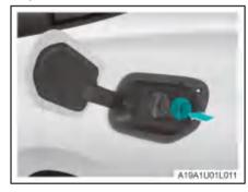
2. Remove the AC charging port dust cap.
