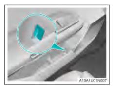
When you cannot open the door from inside in an emergency, you can pull the emergency unlocking device to unlock the door
