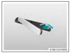
Insert the emergency mechanical key into the keyhole, and turn it to unlock or lock the door.
