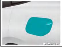
After unlocking the vehicle, press the arrow-indicated area of the charging port cover to automatically open the charging port cover.
