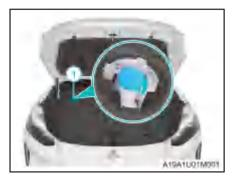
Open the hood, remove the decorative cover 1 , open the washer fluid reservoir cap as arrowed, and check the washer fluid in the reservoir. If the washer fluid level is too low. please add the washer fluid or a mixture of washer fluid and water.
