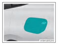
After unlocking the vehicle, press the arrow-indicated area of the charging port cover to automatically open the charging port cover.
