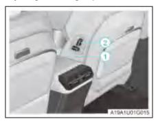
Adjusting the front passenger seat position
