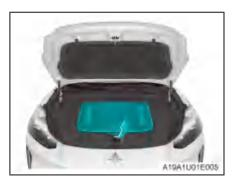
Pull the front trunk release lever upward to open the front trunk.
