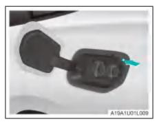
The charging indicator lamp is located inside the charging port, and the status of the charging indicator lamp during charging is as follows.
