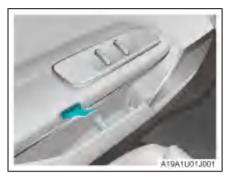
After the door is unlocked, press the door unlocking button to automatically open the corresponding door. (Models with power doors)
