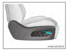
Press the front and rear ends of the front passenger seat legrest adjusting button to adjust the seat legrest. (if available)
