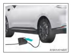
5. Observe the change in the indicated pressure on the tire pressure gauge. When the indicated pressure reaches the standard tire pressure, power off the inflator pump to stop inflating the tire.
