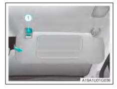
After the sun visor is turned down, disengage it from the fastening hook (1) and turn the sun visor to the side window to block the dazzling light from the side.
