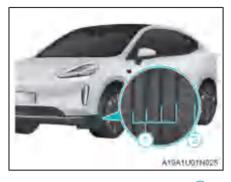
There is a raised "tread wear indicator" (1) on the front of the tire. If the tread pattern wears to the indicator surface, the tire can no longer be used safely and must be replaced immediately.
