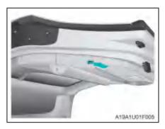
Stand outside the vehicle and press the closing button on the left/right door, and the left/right gull-wing door will close automatically. (Models with rear gull-wing doors)
