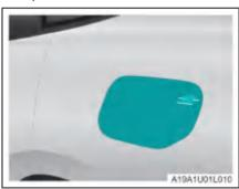
1. After unlocking the vehicle, press the arrow-indicated area of the charging port cover to automatically open the charging port cover.
