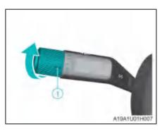
Turn the wiper control knob up or down from the oposition, so that the front wiper position icons are aligned with the wiper control knob position reference icons 1 in turn, and the front wiper mode can be selected. The specific control is as follows:
