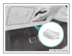
The OBD DLC is located at the lower rear of the instrument panel. Data such as the VIN and vehicle status information can be read by connecting a special diagnostic scan tool to the OBD DLC.
