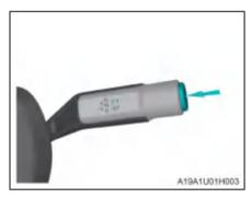
After the vehicle comes to a full stop, press the "P" button to shift to "P" gear. Then the EPB is automatically enabled.
