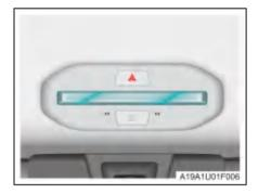
○ Touch the front reading lamp cover to turn the front reading lamp on or off.
