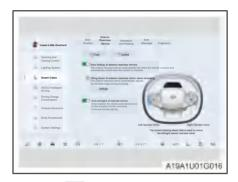
Touch the A button on the center console display to enter the exterior rearview mirror adjustment interface, turn the roller on the steering wheel or touch the steering wheel direction adjustment arrow on the center console display to adjust the exterior rearview mirror to a suitable angle.
