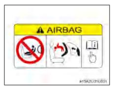
Please follow the warning label on the sun visor: Do not install a child restraint system on the front passenger's seat.
