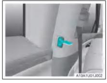
After the door is unlocked, press the door opening button on the left/right B-pillar to automatically open the left/right gull-wing door. (Models with rear gull-wing doors)
