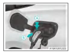
While pressing the charger button in the direction of arrow A, unplug the charger in the direction of arrow B.
