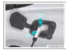
7. While pressing the discharger button in the direction of arrow A. unplug the discharger in the direction of arrow B.
