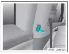
After entering the vehicle, press the door closing button on the left/right B-pillar and the left/right gull-wing door will close automatically. (Models with rear gull-wing doors)
