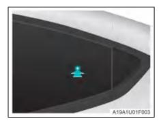
Unlock the vehicle, press the left/right door switch, and the left/right gull-wing door will open automatically. (Models with rear gull-wing doors)
