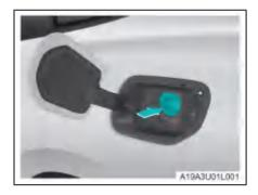
Remove the AC charging port dust cap.
