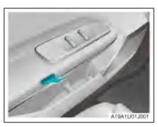
The locked door can be unlocked by pressing the door unlocking button.
