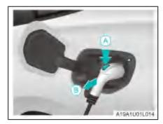
While pressing the charger button in the direction of arrow A, unplug the charger in the direction of arrow B.
