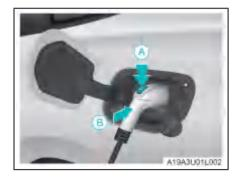
3. While pressing the button of the charger in the direction of arrow A, insert the charger in the direction of arrow B. After the charger is successfully connected, the vehicle charging indicator lamp stays on in yellow, and the charger indicator lamp on the instrument comes on.
