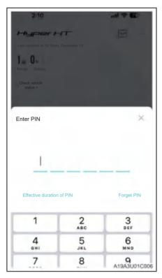
3. After the setting is completed, the PIN input interface will pop up. Enter the PIN, and the vehicle will perform the vehicle control operations you desire.
