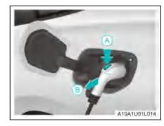
While pressing the discharger button in the direction of arrow A, unplug the discharger in the direction of arrow B.
