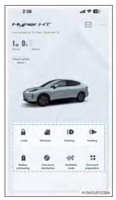
After the vehicle is successfully linked to the account, the vehicle can be remotely controlled on the intelligent vehicle control interface.
