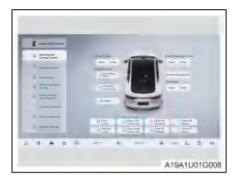
When a child takes a rear seat, please activate the child safety lock on the corresponding side through the center console display before closing the door. At this time, the door cannot be opened from inside, so as to prevent the child from opening the door unexpectedly.
