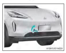
2. Insert the towing hook into the towing eye, turn it clockwise and tighten it.
