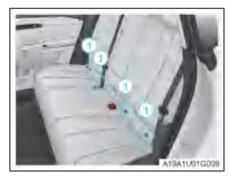
There are four ISOFIX/ISIZE anchorages provided between the rear seat back and the rear seat cushion for installation of child seat. Label 1 is used to indicate the position of ISOFIX anchorage.
