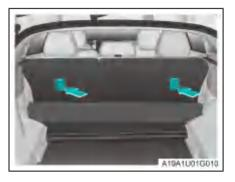
The LATCH anchorage is located on the back of rear outboard seat.
