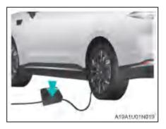
4. Start the vehicle, and turn on the power switch of the inflator pump to start inflation.
