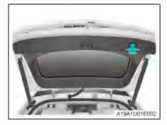
When the trunk lid is open, press the closing button on the trunk lid to automatically close the trunk lid.
