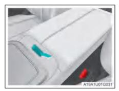
Press the storage box lid unlocking button to open the central armrest box.
