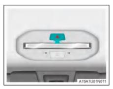
If the vehicle is faulty or involved in a traffic accident, please turn on the hazard warning lamps to alert other vehicles.
