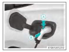
While pressing the button of the discharger in the direction of arrow A, insert the discharger in the direction of arrow B.
