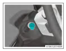
Press and hold the front wiper washer button to have the front washer nozzle spray washer fluid. After the wiper control lever is released, the front washer nozzle stops spraying the washer fluid, the wiper operates several times, and then operates once after a period of time and stops.
