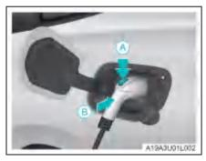
3. While pressing the button of the discharger in the direction of arrow A, insert the discharger in the direction of arrow B.
