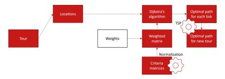
Figure 13: Visualization of model NewTour: new tour generation
